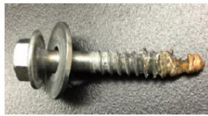
During the installation process for a garage door, a Tek Screw being used to attach door components, struck a live electrical cable causing sparks and shorting out the power to the electrical supply to the house causing a burn mark on the wall.
